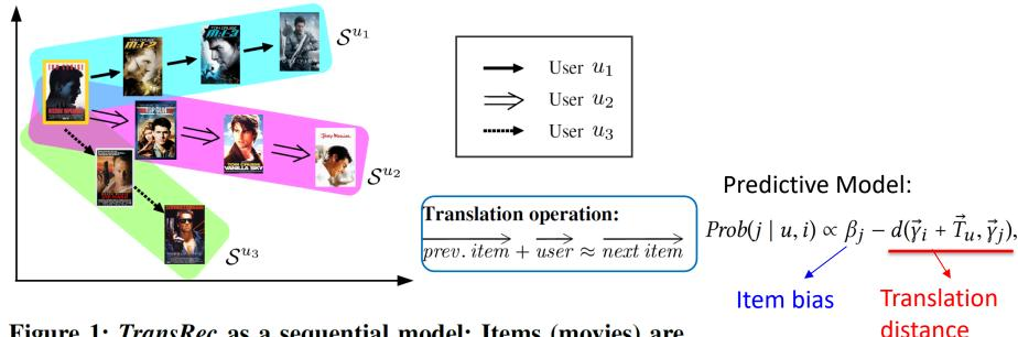
Figure 1: *TransRec* as a sequential model: Items (movies) are embedded into a 'transition space' where each user is modeled by a *translation* vector. The transition of a user from one item to another is captured by a user-specific translation operation.
