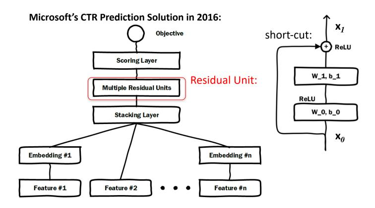
The main difference from Wide&Deep is the use of residual layers, which allow deeper network to be built (~10 layers).
