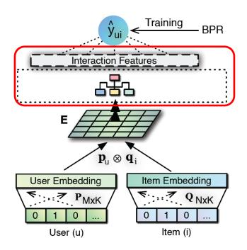
Above the interaction map are hidden layers, which aim to extract useful signal from the 2D interaction map.
